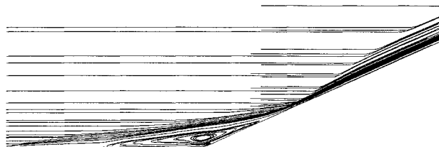
Fig. 3 Streamlines for flow past 24-deg compression corner, USA-PG2 solution.
